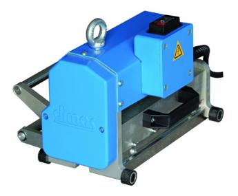
The DIPRO-SRT crimping machine creates crimp profile n° 1 in a single run.
